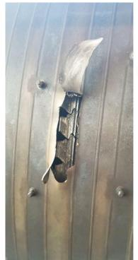
Power Turbine rotating blades pushed through casing
